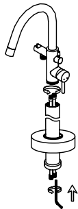
4. Connect body by H8 screw tool, install the decorative cover from top of the pipe, tighten up inlet pipe to the body with H8 hex key.
